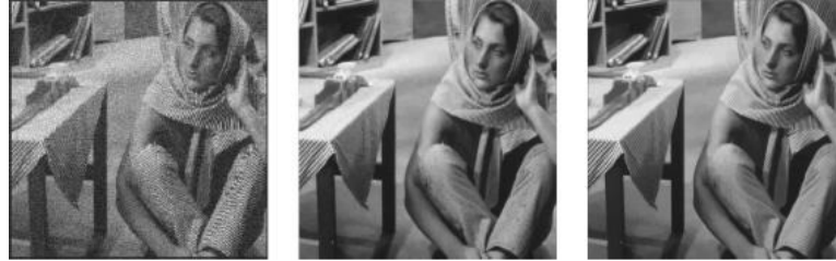
FIGURE 14. Left: noisy Barbara image, middle: restored image by TV with L^1 -fidelity term, right: restored by the proposed model
