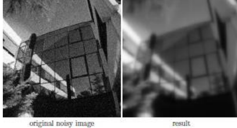
FIGURE 1. Restoration of the noisy “Borel building” image (additive Gaussian noise) edges are lost.
