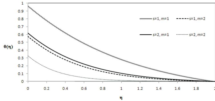
FIGURE 3. Temperature profiles for different  $s$ .
