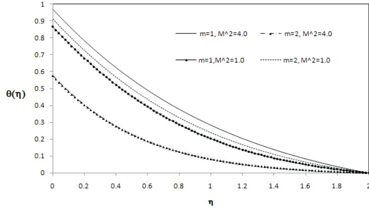
FIGURE 5. Temperature profiles for different M.
