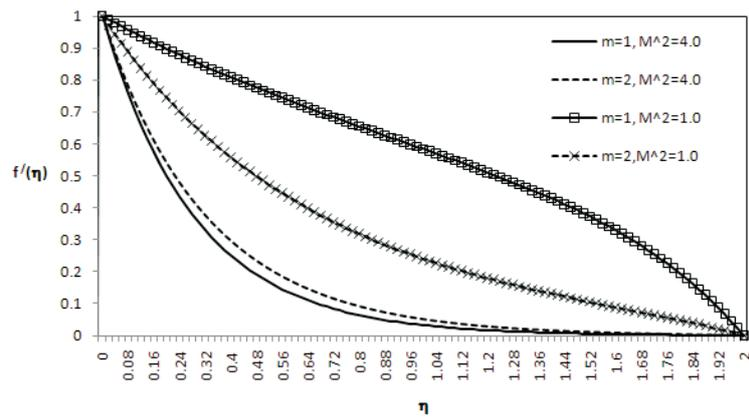
FIGURE 4. Velocity profiles for different  $M$ .
