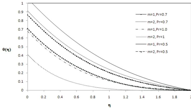
FIGURE 6. Temperature profiles for different Pr.
